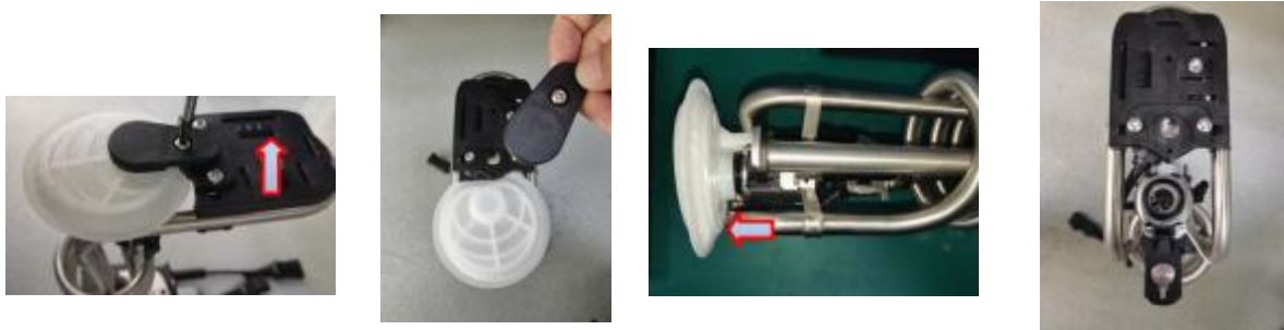
Fig. 5-2~5-5 Removal Process of the Urea Filter Bag
