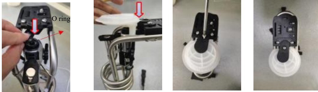
Fig. 5-6 ~ 5-9: Installation Process of the Urea Filter Bag
