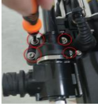
Fig. 2-19: Locations of the Four Screws on the Solenoid Valve for Water and Power Cut-off
