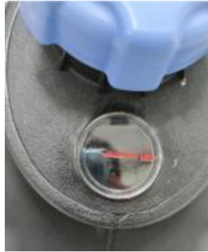
Fig.5-1 The position of the maximum fill line
