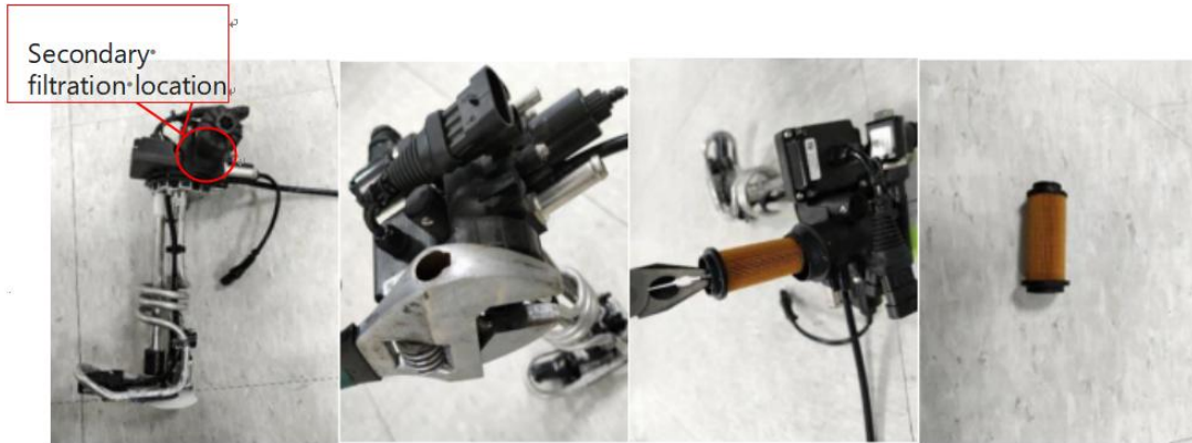
Fig. 5-10 ~5-13: Disassembly Process of the Secondary Filter
